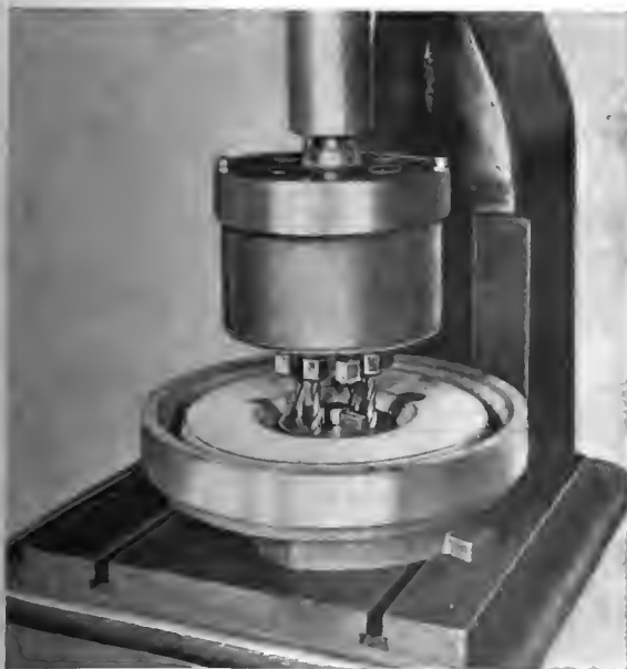
E—Convincing Example of the Cluster Box Idea in Which the six Flange Bolt Holes of the Flywheel are Drilled Simultaneously, Using a Single Spindle Drill Press for the Purpose
